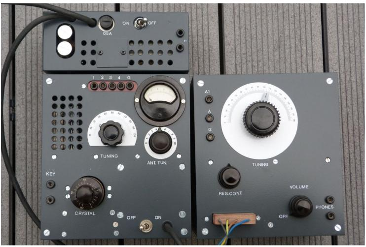
German Abwehr spy set from WW2. Transmitter crystal controlled using AL5 tube and built in mains supply. Receiver E75, regenerative 1-V-1 with 3x CF7 and PSU GLE85. The transmitter is able to double the crystal frequency
