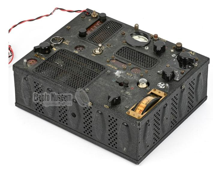
Manufactured by the Marconi Company in the UK in 1944, close towards the end of WWII. It was intended for clandestine operations on occupied territory, by agents, special forces and resistance units. The transceiver came as a replacement for the rather bulky Type 3 Mk.II (B2) Operating between 3 and 9 Mc/s, RX was superhet using 7Q7 and two 7H7 valves (IF 1.2 Mc/s) TX had a max. of 5 W and used 7H7 and 7C5 valves. PS could use all mains voltages and 6V DC
