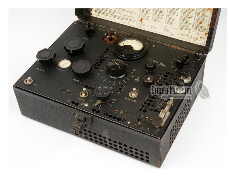
Developed during WWII by Tadeusz Heftman of the Polish Military Wireless Unit (Polski Wojskowy Warsztat Radiowy) in Stanmore (UK) Operated from 2-8 Mc/s with an output of 50 W CW, a later BP-5 employed an AM modulator. RX was superhet using 6K8 6Sk7 6SQ7 and 6SC7 TX used 6V6 and 629, also used by SOE it was considered better than UK counterparts
