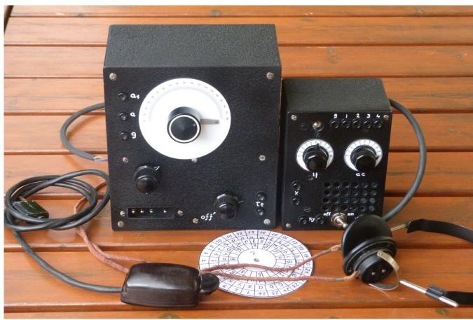
Wulf Schmidt, a double-agent known mainly with his alias "TATE" used this set. The TATE radio is the only set known when the Abwehr combined the transmitter S88 with KL2 tube (2W) and the wartime German Abwehr standard receiver as a special version using 3x KF4 battery tubes instead of the usual 3x CF7.
