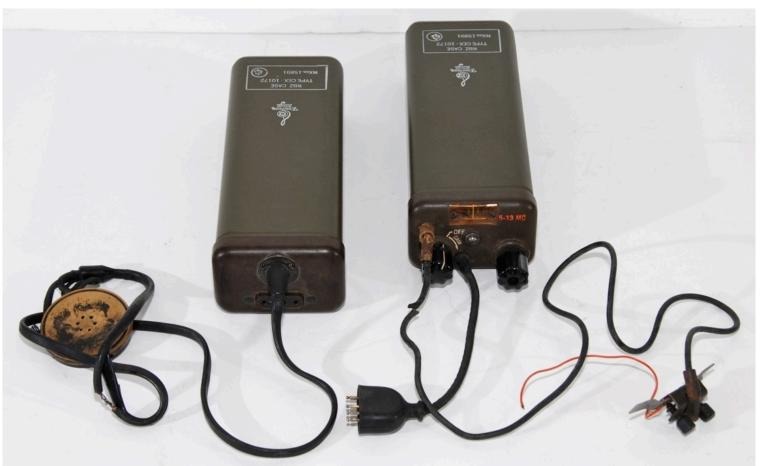
The US was rather late to the game, this was a miniature tube receiver (1T4 RF, 1R5 OSC/MIX, 1T4 IF, 1S5 det, and 1L4 AF. Covered 2-5.8 Mc/s later extended to 13 Mc/s, used in D day landings and some raids, mostly dropped behind lines for Resistance to listen to BBC.
