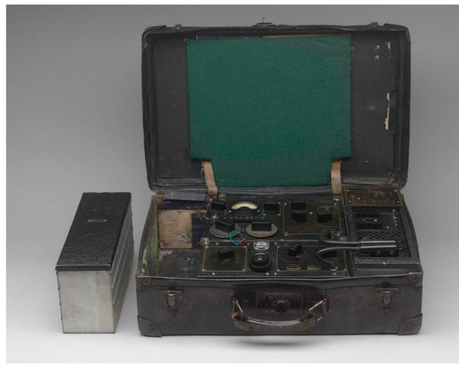
Manufactured by the **Radio Communication** Department of the SOE at Stonebridge Park. The transmitter was crystal controlled and used an EL32 for the MO and a 6L6 for the PA, it covered 3 to 16 Mc/s in 7 bands. The receiver covered 3.1 to 15.2 Mc/s using two tubes, a 7Q7 and 7R7. The Power supply could accommodate all possible mains voltages as well as 6 V DC
