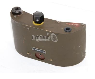
The S-phone was a two-way full-duplex UHF radio system, developed in 1942 in the UK, for use by the Special Operations Executive (SOE) during WWII. It was used by resistance groups and SIS agents operating behind enemy lines, for communication with intelligence officers in airplanes, flying close to the occupied territory at high altitude. The S-Phone consisted of a ground unit and a matching airborne unit. The ground unit is also known as Type 13, Mk II, Mk III or Mk IV
