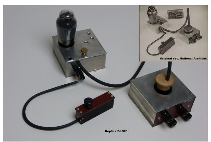
This tiny box tried to solve the bulkiness of spy radios. The principle is simple: All you needed was a normal domestic radio with a known final tube for the audio of the radio, unplug the final tube, insert the adapter plug instead and put the tube into the adapter. All voltages were obtained from the radio, the AF tube is now used in a RF power oscillator.
