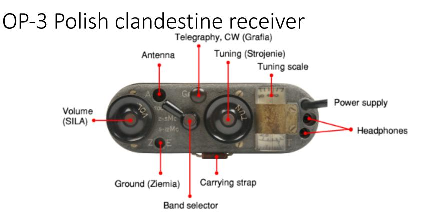
This was a portable clandestine receiver, developed and built during WW-II by the Polish Military Wireless Unit (Polski Wojskowy Warsztat Radiowy) in Stanmore (UK). The receiver was introduced in 1943 and was intended for the reception of the BBC and Polish Radio Broadcasts from London. It is also known as Type 30/1 and was sometimes used as backup for clandestine radio sets.
