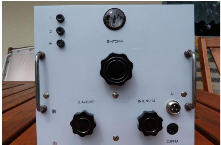
Employed: 3x EF6 tubes regenerative design: preamp, detector and AF stage (1-V-1) 6,0-14,4 MHz Magnifier lens scale. RRN-3 plus the transmitter TRN-3 forms the set RN-3, the Italian version of the German SE 85/14.
