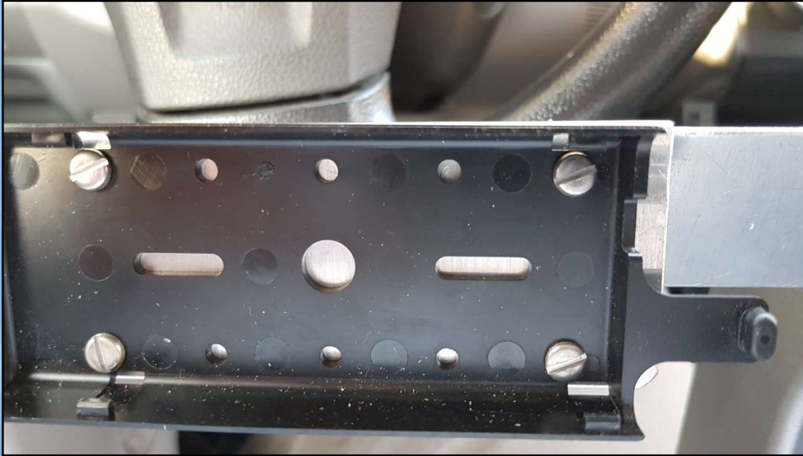
Control head mounting shell on bracket
