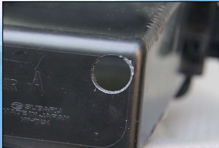
Hole in bin for control, microphone and speaker cables
