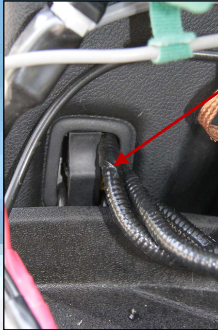
Bonding cables to car body
