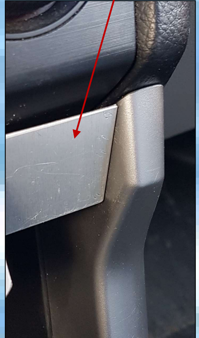
Control head mounting bracket
