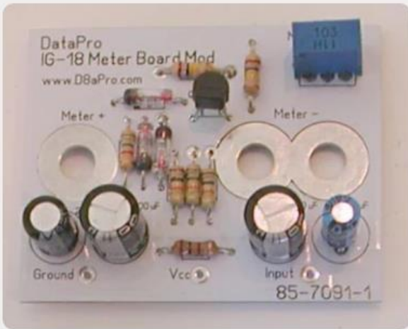
THD Improvement kit for IG-18 series audio generator test equipment (meter buffer board ONLY) - IGA-18-2
