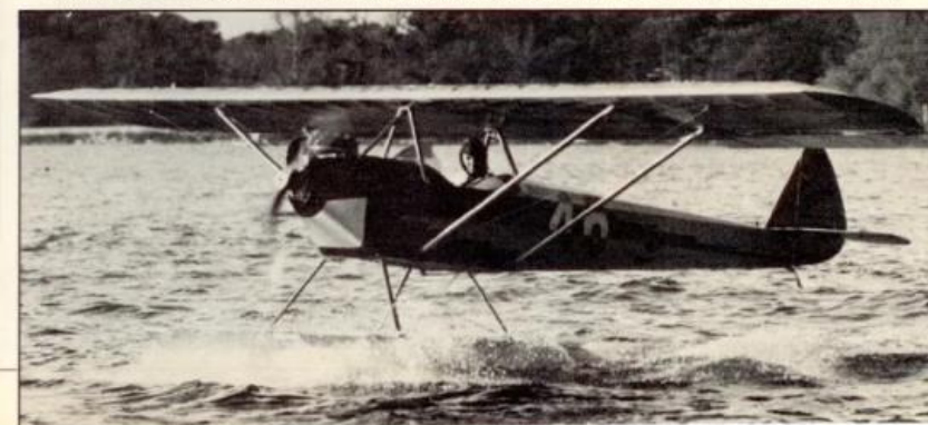
A pair of early Heath Parasols is shown above. The 1925 prototype, back, has the thin-section Thomas-Morse wing. Subsequent models used the Clark-Y airfoil. The Parasol below is equipped with flat-bottom wooden floats. Until modern ultralights, the Parasol was probably the lightest floatplane ever built.
