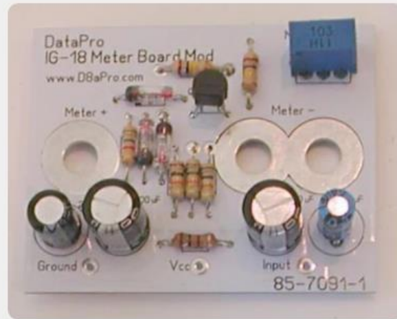
THD Improvement kit for IG-18 series audio generator test equipment (complete kit) - IGA-18-1
